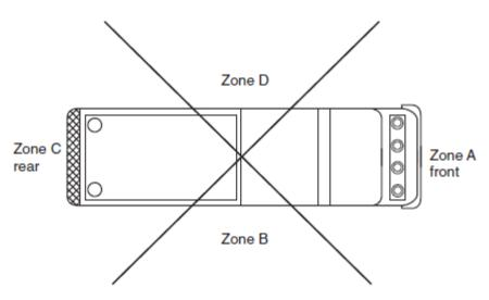
Figure 13.8.3.2 Warning Zones for Optical Warning Devices
