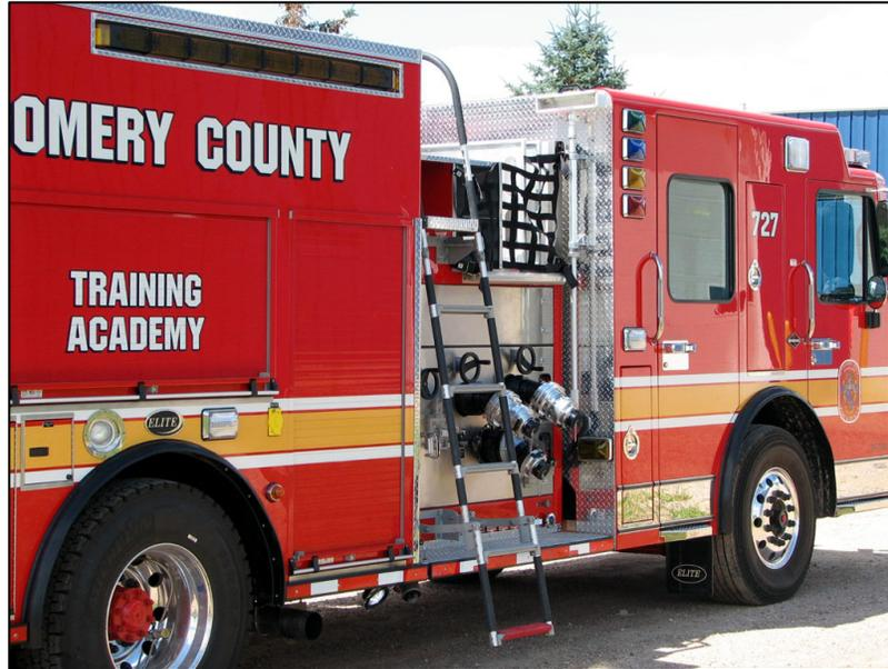
Figure 15: MCFRS apparatus outfitted with an arrow board on the side of the vehicle (at left of photo above the county lettering). Photo credit: Montgomery County (MD) Fire and Rescue Service
