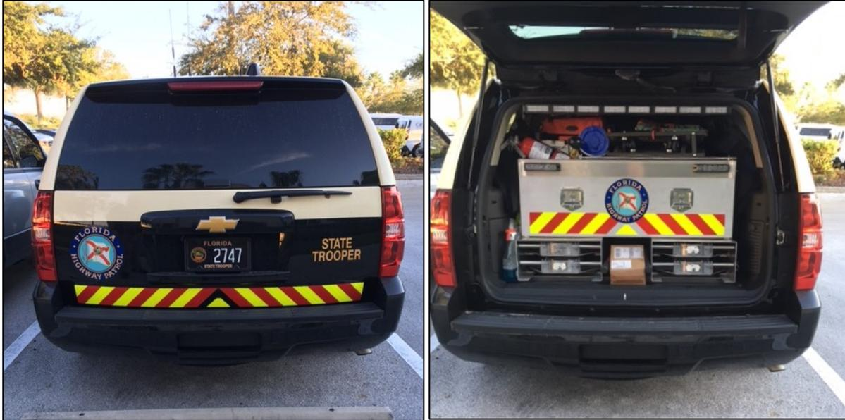
Figure 9: Florida Highway Patrol SUV with conspicuity markings inside and outside the liftgate. *Photo credit: Florida Highway Patrol.*
